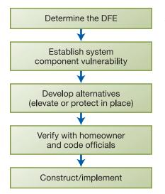
Figure 5W-4. Wet floodproofing of utilities design process
