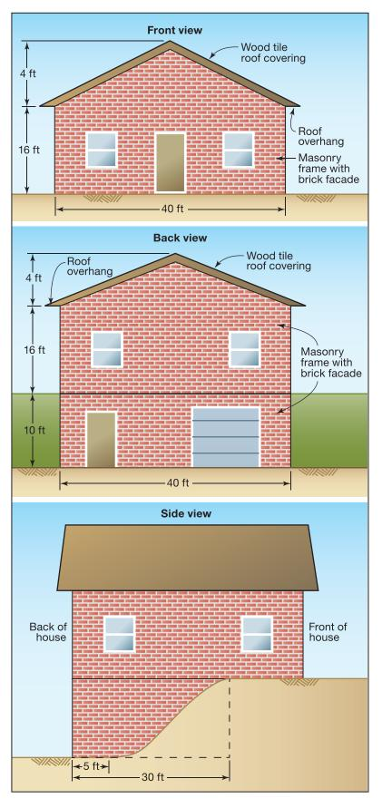
Figure 6-31. Elevation drawings from the front, back, and side of the Borges house
